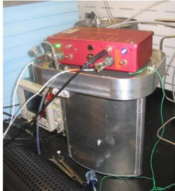
Figure 1. VCSEL hygrometer sealed up in the stainless steel housing for calibrations
