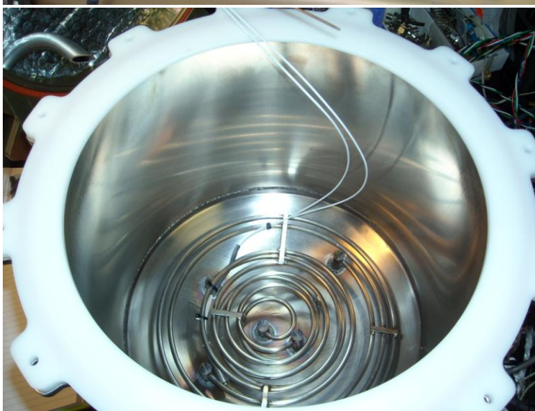
This photo shows the LN 2 heat exchange coils at the base of the dewar, this is where N 2 gas is cooled prior to flow into the organic removal traps.
