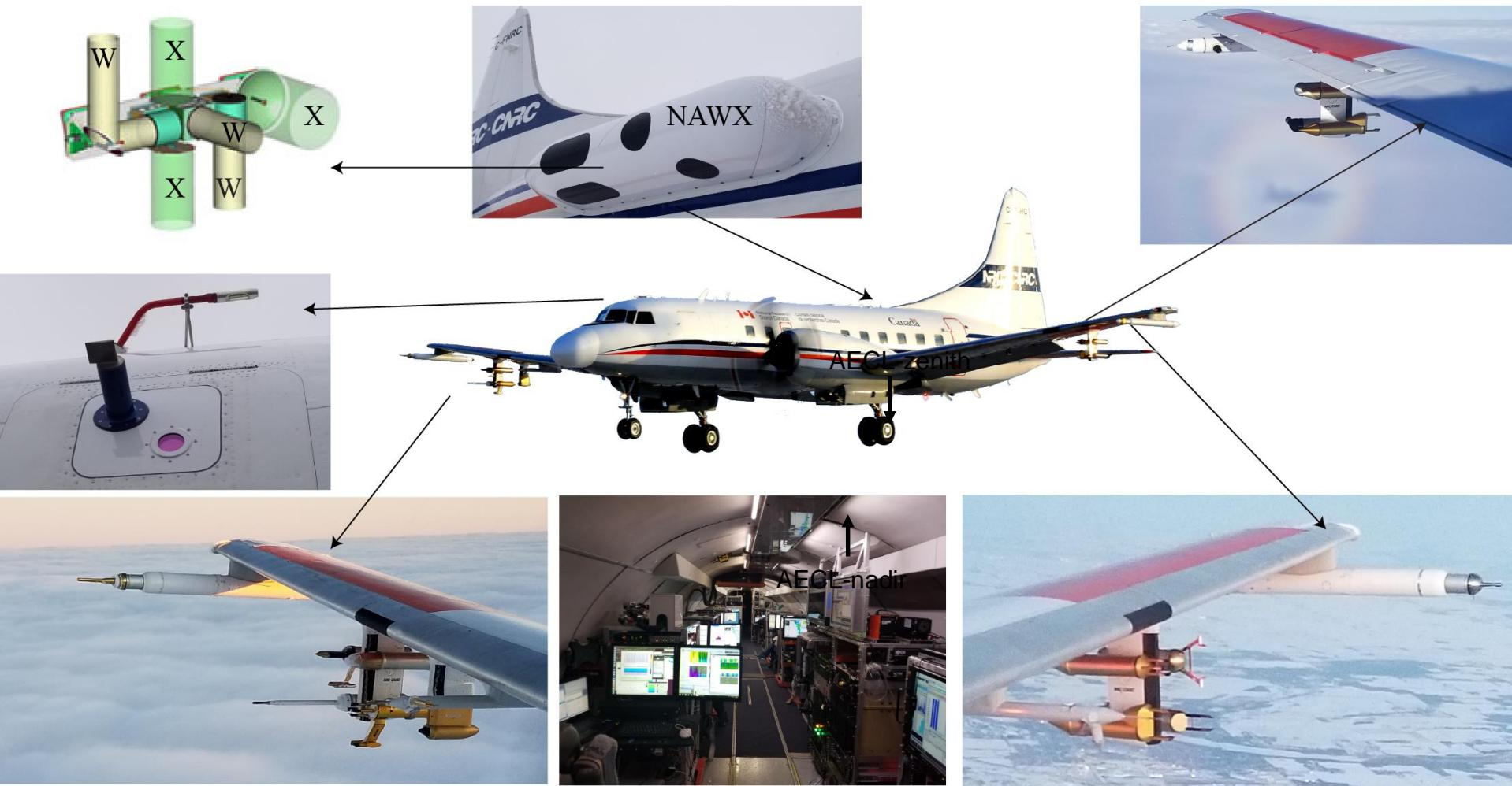
Extensive in-situ and remote sensing capabilities for measurements of atmospheric state, compositions (aerosol, cloud and precipitation – type, size, phase and bulk properties).
