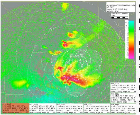
Grid of radars provide ~ 100km X 120 km dual-Doppler area with overdetermined sampling
