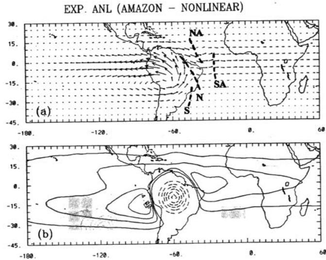
Fig. 14: 500 mb  $\omega$  in a dry primitive-equation model including topography, in response to a specified, realistically strong, deep convective heat source over Amazonia. Solid contours (interval  $1 \text{ hPa } d^{-1}$ ) indicate subsidence. Dashed contours (interval  $20 \text{ hPa } d^{-1}$ ) indicate forced ascent over the heating region (Gandu and Silva Dias 1987).
