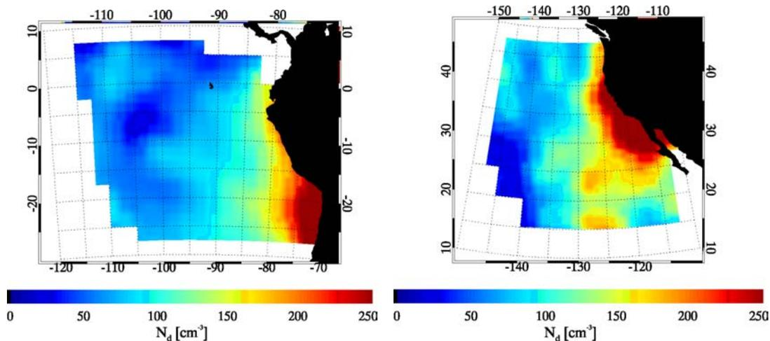
Fig. 5: MODIS retrievals of mean cloud droplet concentration for Sept.-Oct. 2000-2001. Regions of broken cloud cover or cloud above 2 km elevation are excluded (Rob Wood).
