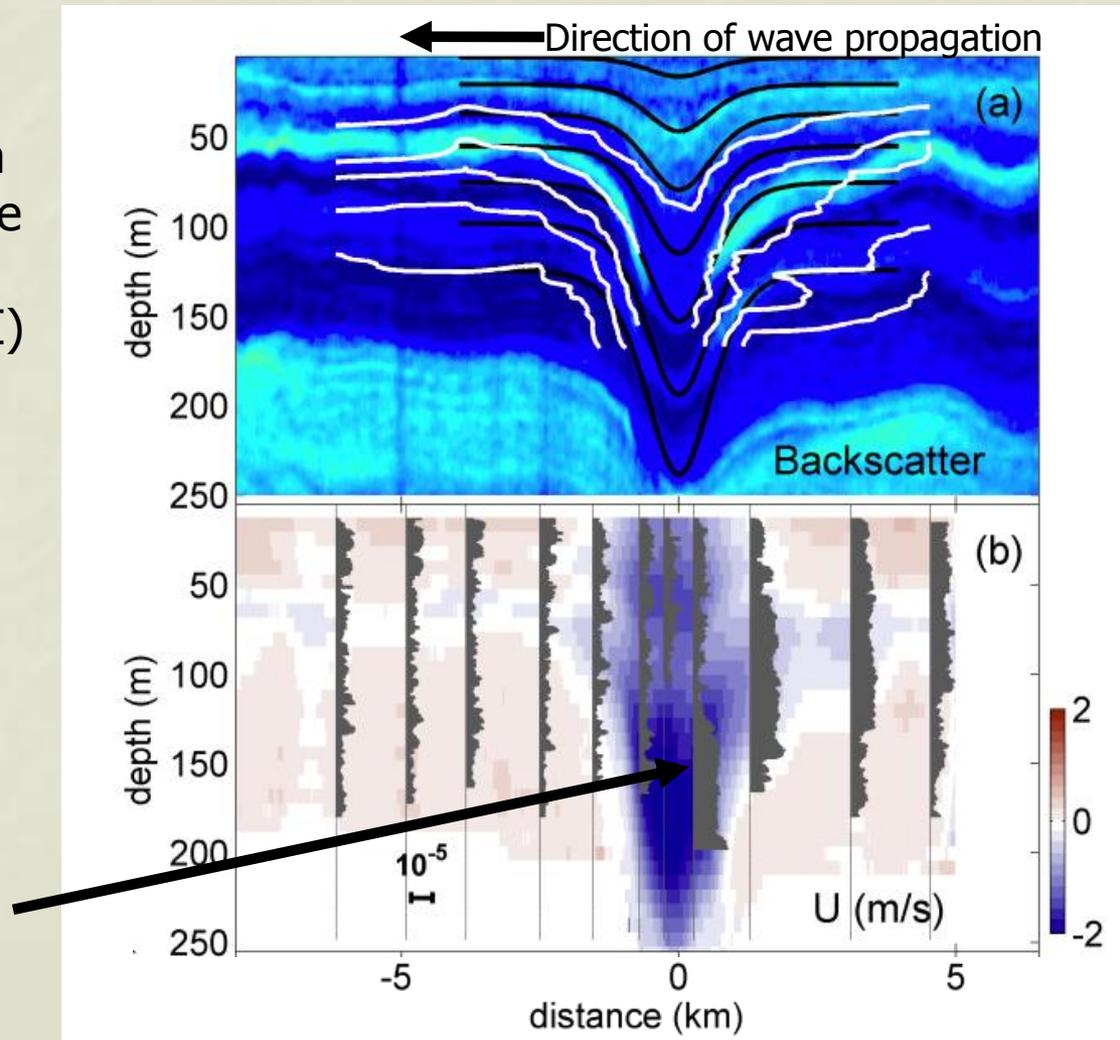
The very large dissipation ( $\sim 10^{-4}$  W/kg) observed in and behind the wave is important to the evolution of the wave
