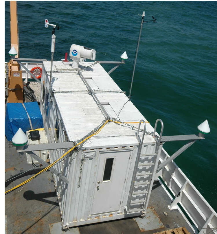
HRDL Mounted on the Fantail of the RV Ron Brown during TEXAQS 2006
