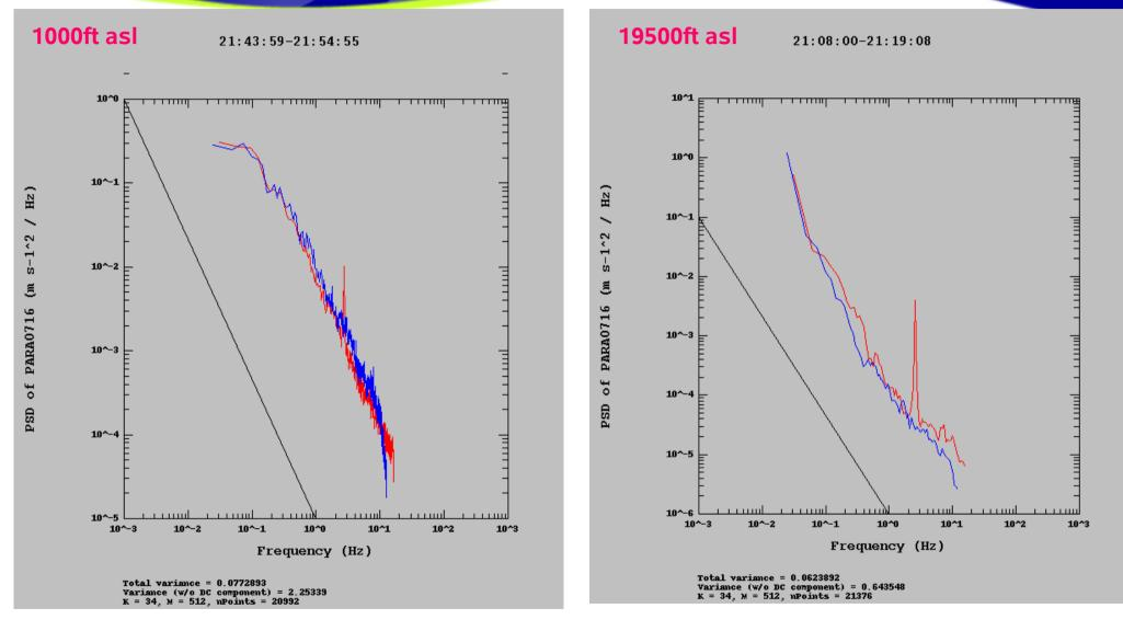
BAe146 data contain a spike at around 3Hz which is derived from noise or aliassing in INU attitude-rate data
