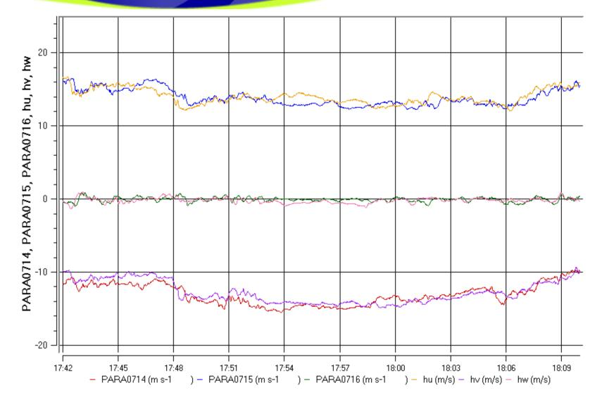
These measurements were obtained on racetrack legs during which the 146 was overtaking the King Air
