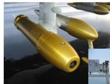
AMAX-DOAS pylon on the Gulfstream V aircraft in H
