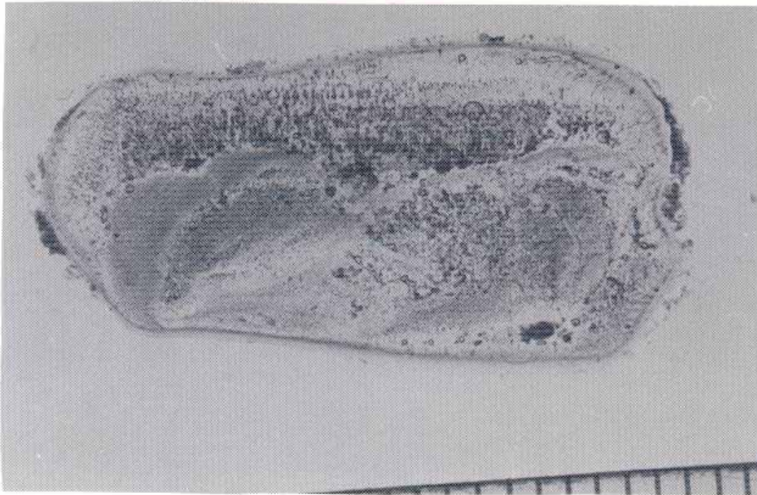
Figure 1: Photograph of thin-section of hailstone caught during the seventh penetration of Flight 545 on 1 June. Bubble-filled layer in upper two-thirds of photo may be water frozen onto the particle after capture. Partially-visible scale at bottom is graduated in millimeters. [Thin-section preparation and photo courtesy of Dr. Charles A. Knight, National Center for Atmospheric Research]
