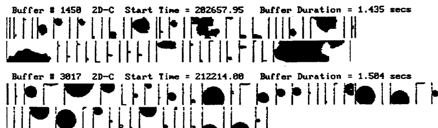
Fig. 3: Sample images from 2D-C probe for Penetration 2 near -11^\circ\text{C} (upper) and Penetration 7 near 0^\circ\text{C} (lower). Vertical bars represent about 1 mm.
