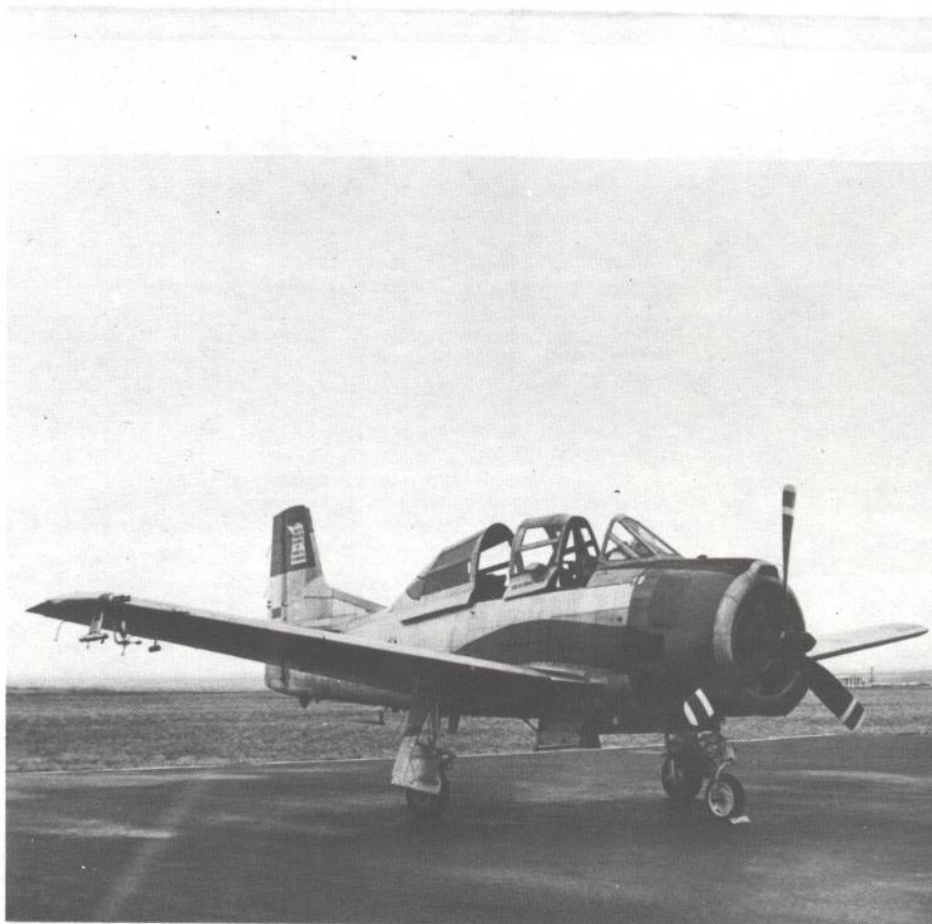
Fig. 1. The armored T-28 hail research aircraft.
