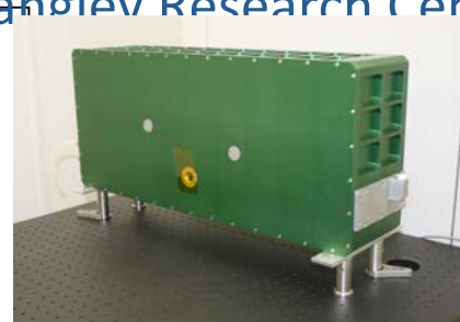
DAWN Transceiver (Transmitter + Receiver) 250 mJ/pulse, 10 pulses/sec. 5.9" x 11.6" x 26.5", 75 lbs. (no telescope or scanner)
