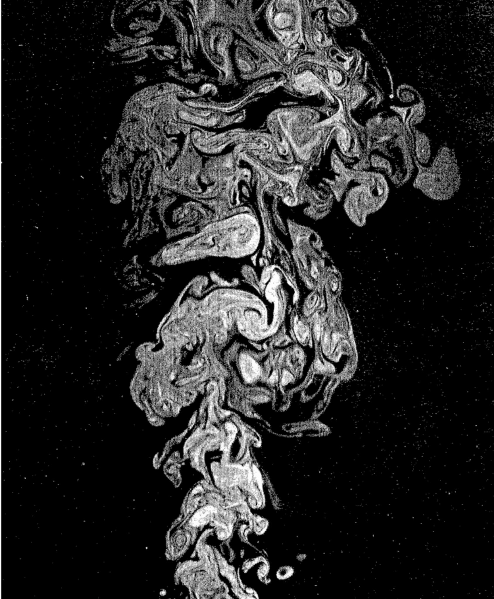
LES of passive scalar in a convective boundary layer
