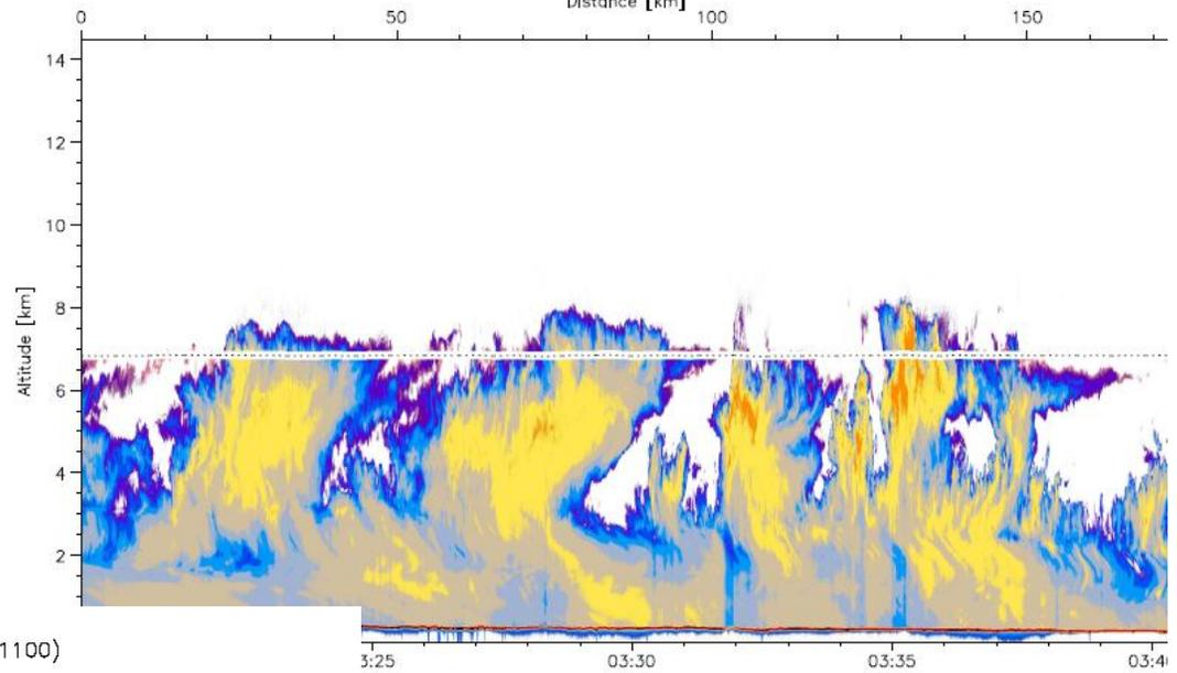
Below: Wyoming Cloud Radar reflectivity-flight occurred Dec 03, 2009. Radar returns appear to contain upright (vertical) convective structures.
