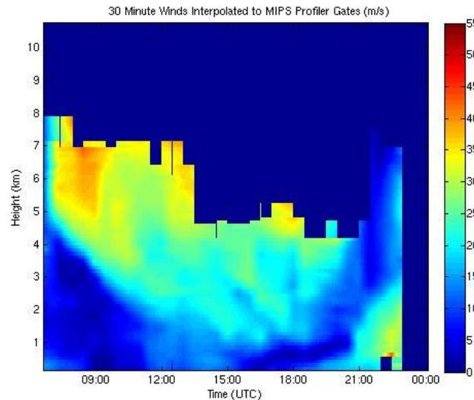
Analyzed winds interpolated in space and time to profiler gates for the RUC (top left), MIPS (bottom), and UMO Soundings (top right) for IOP1. Dark blue areas indicate missing data.
