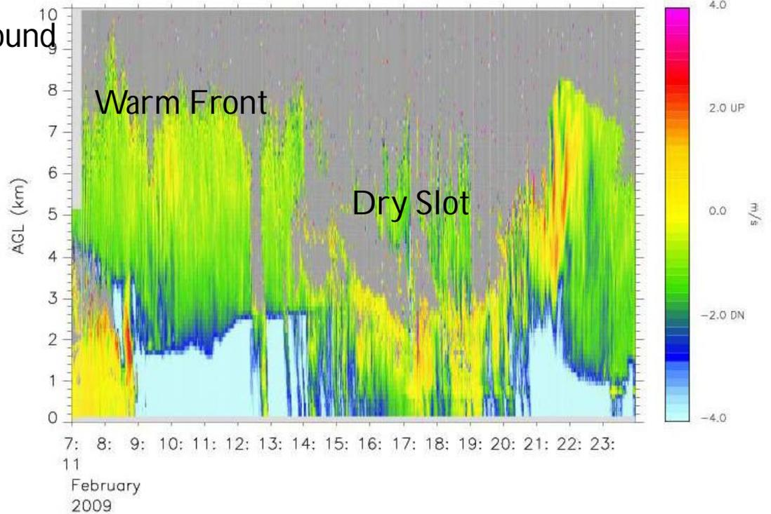
MIPS profiler SNR (top) and radial velocity (bottom) from IOP 1. Especially noteworthy is the area on the edge of the wraparound region that shows positive radial velocity measurements.
