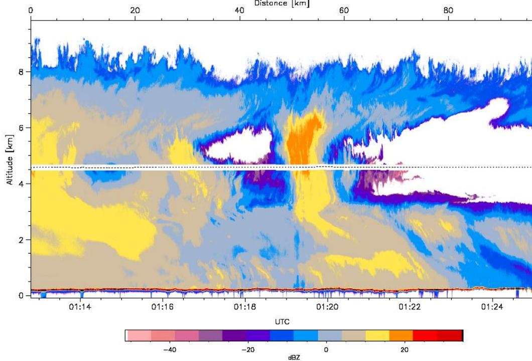
Above: WCR reflectivity from Dec 9, 2009. Convective structures again are evident throughout the flight path.
