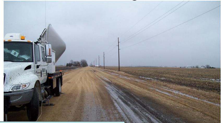
Some beam blockage is unavoidable, particularly with powerlines present along many roads. Where possible, sites have been chosen such that blockage is in less critical directions.
