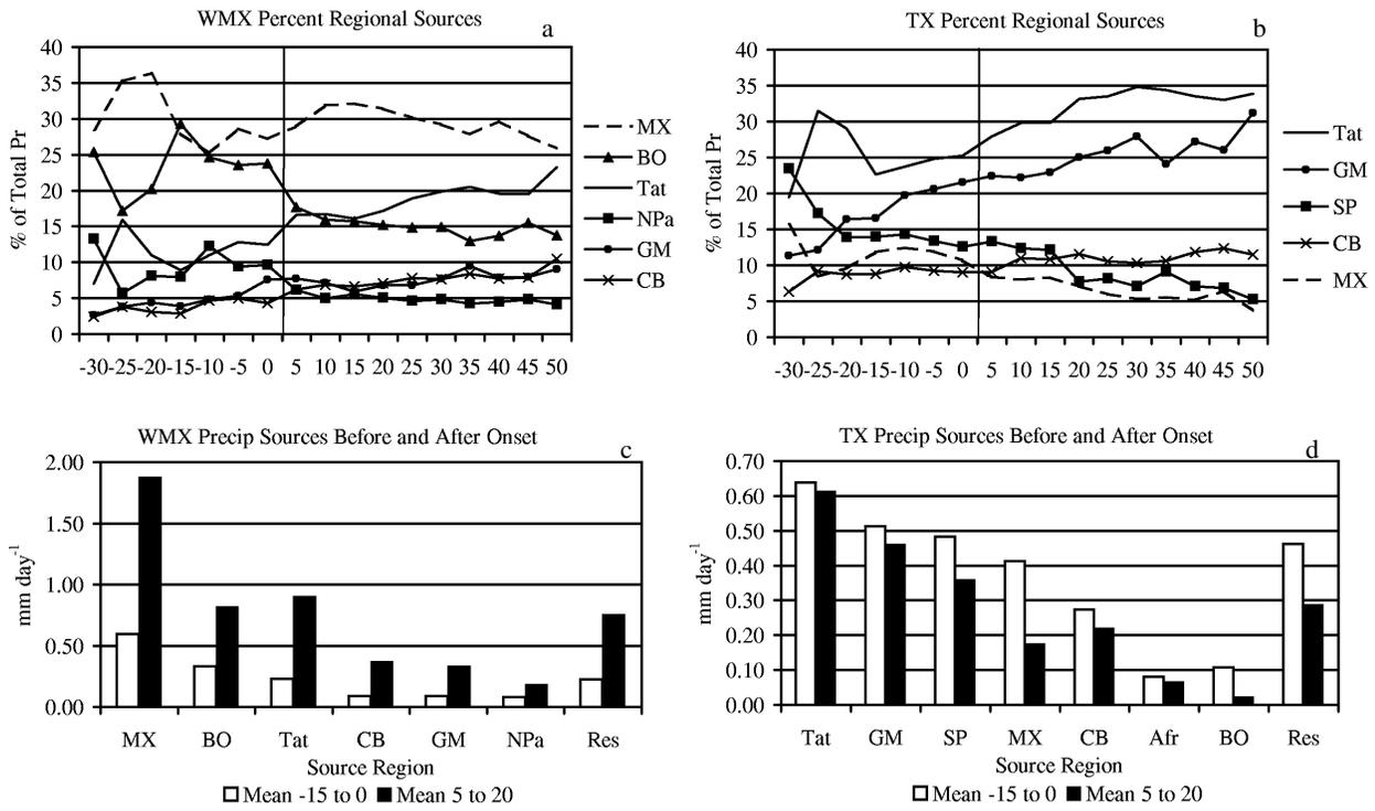
**Figure 10.** WVT data before and after WMX monsoon onset. Composite time series of percent of total precipitation for the major water sources in (a) WMX and (b) TX. WVT precipitation amounts of the major water sources before and after WMX monsoon onset for (c) WMX and (d) TX.
