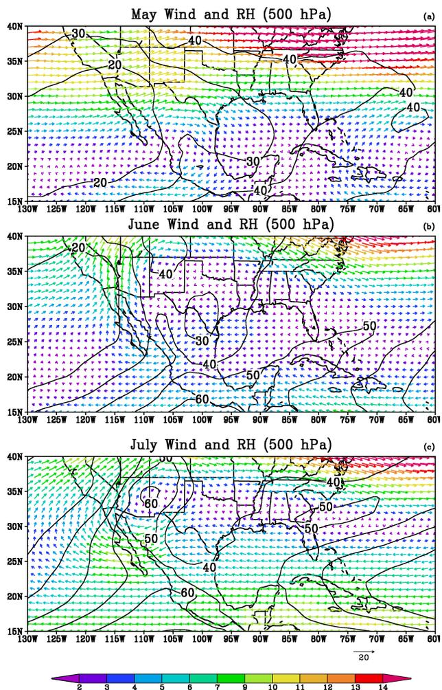
**Figure 4.** 500 hPa 15-year mean wind and relative humidity fields for (a) May, (b) June and (c) July. Wind vectors are colored by the magnitude of wind speed ( $\text{m s}^{-1}$ ) and relative humidity contoured by 10 % intervals.
