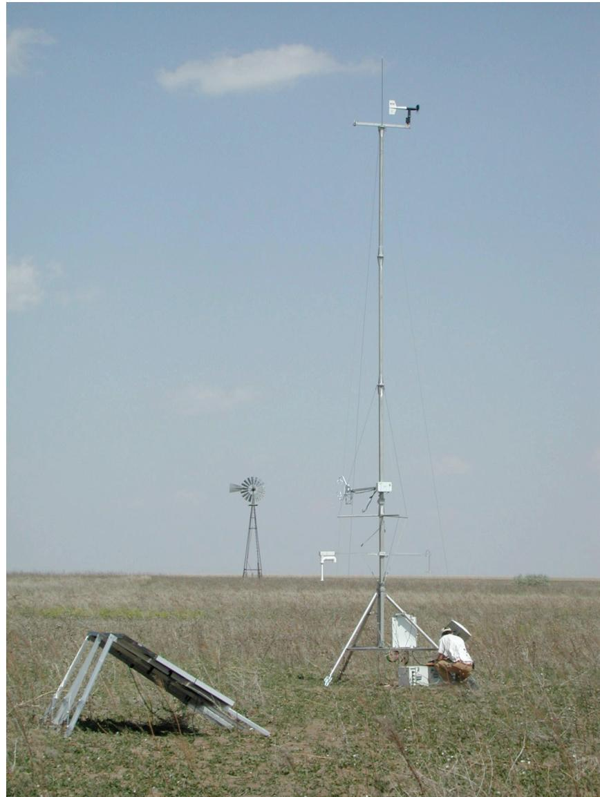
ISFS is a configurable suite of towed sensors, commonly used to study exchange processes between the atmosphere and the earth's surface.
