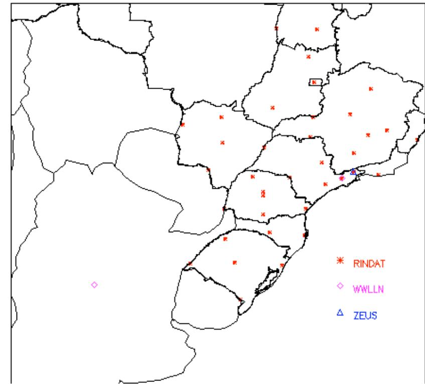
Position of the lightning sensors that operate in real-time over South America. The Brazilian lightning detection network (RINDAT) is defined in red (48 sensors), the World Wide Lightning Location Network (WWLLN) in purple (3 sensors) , and ZEUS lightning monitoring system in blue (2 sensors)
