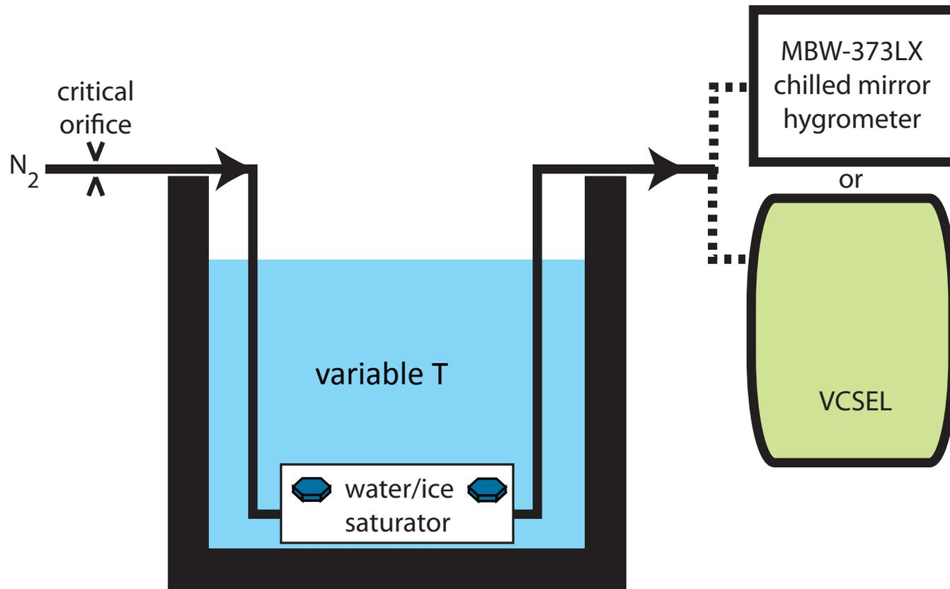
saturate "dry" nitrogen in 1 L volume, 200-1000 sccm flows (bath  $-85$  to  $+20^\circ\text{C}$ )
