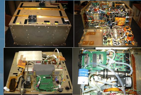
**NWAS:** (NOAA Whole Air Sampler) 20 lb. per 12 flask pkg., 2 to 4 NWAS pkg per flight, 6 in rack.
