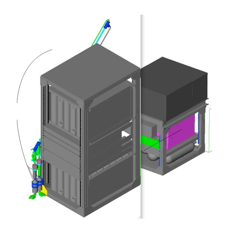
PANTHER: (PAN and other Trace Hydrohalocarbon ExpeRiment,) 200 lb., 6-channel GC (gas chromatograph).
