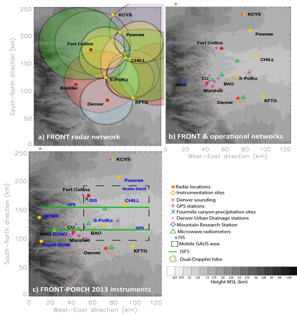
Figure 6: FRONT radar network and surface instruments for the FRONT-PORCH 2013 experiment. a) NSF FRONT radar network including the WSR-88D weather service radars at Denver, CO and Cheyenne, WY. Dual-Doppler lobes are indicated in color. b) FRONT and existing hydrometeorological and humidity stations in the CFR domain. c) FRONT-PORCH instrumentations with requested NSF facilities indicated in blue. The basic orientation of the surface instrument transects are shown with a green line.
