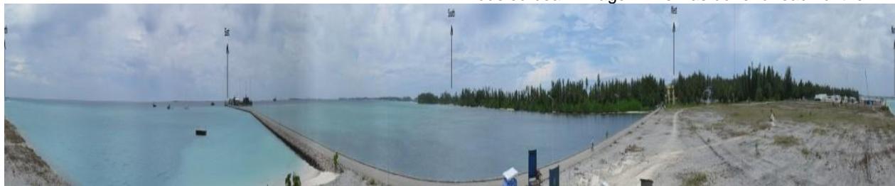
Fig. 2: Panoramic image taken from the S-Pol pedestal, 3 m below the center of the dish; north is at each edge, and the vertical scale has been exaggerated by a factor of four to better show variations in the blockage.
