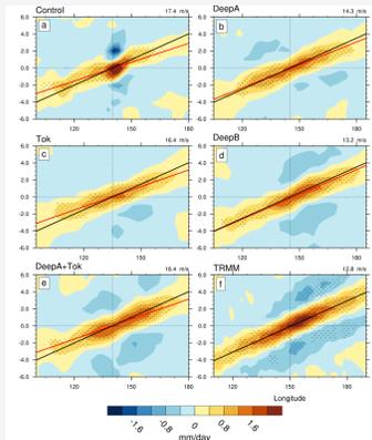
Fig 5. Lagged regression of equatorial precipitation (10°S-10°N) onto a Kelvin wave index at the point of maximum Kelvin wave variance indicated by the vertical line. The black line indicates a least squares estimate of the propagation speed estimated from TRMM and the red lines are that for each simulation. Stippling indicates significance at the 95% level.
