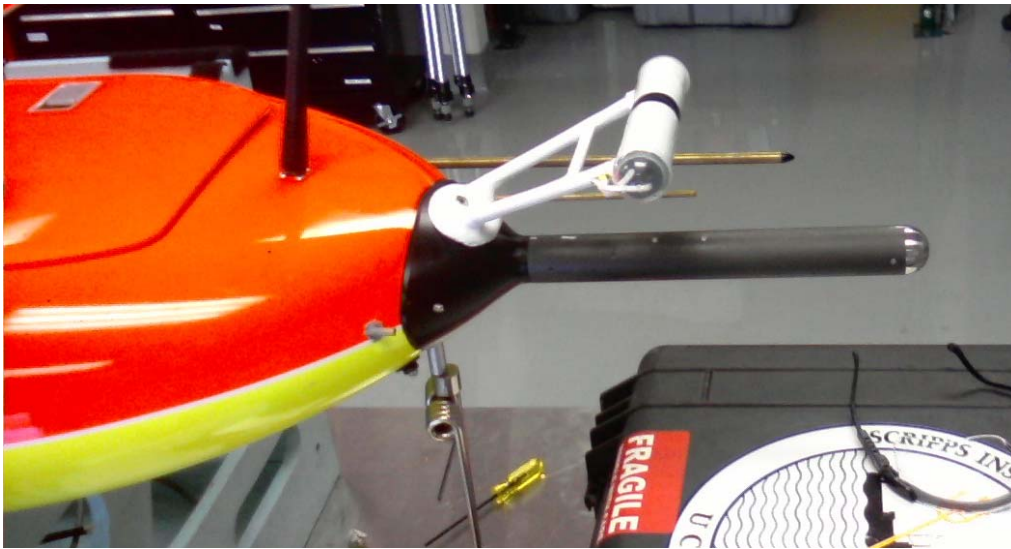
Figure 4: Krypton hygrometer collocated with 9-port turbulence probe mounted on a BAE Manta C UAS.
