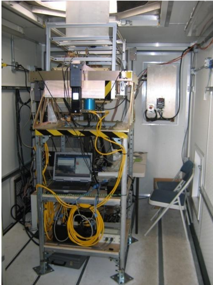
Radar and Stabilizer in seatainer during VOCALS 2008
