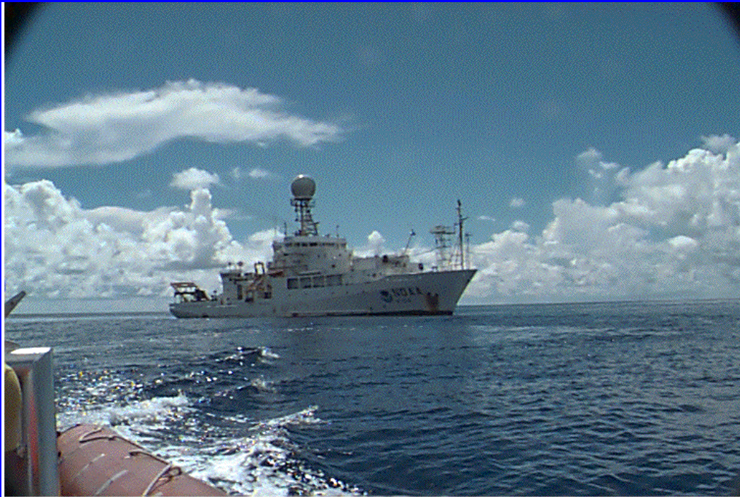
Figure 2: Picture of NOAA's R/V Ronald H. Brown taken from the Rugged-Hull Inflatable Boat, which was returning from a successful sphere calibration exercise. The radome atop the ship shows the location of the C-band Doppler radar.
