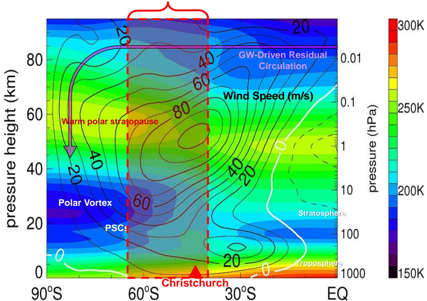
**New DEEPWAVE instruments will provide sensitivity to the dominant GW scales relevant to quantifying GW influences and parameterization needs**
