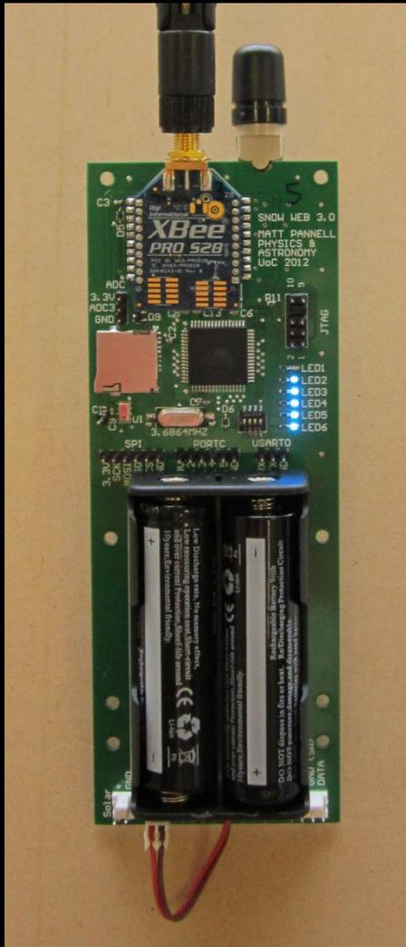
Our capability in hardware development has allowed us to develop an expandable Zigbee-enabled environmental monitoring system.
