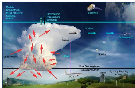
The DC8 payload included the ISAF and the Difference Frequency Generation Absorption Spectrometer (DFGAS) to measure HCHO from storm inflow and outflow, providing ample comparative opportunities for instrument validation.
