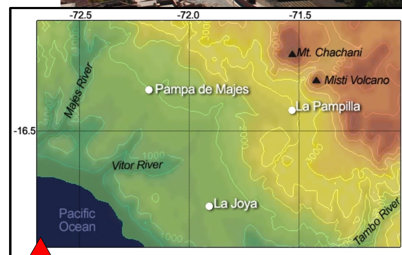
Fig. 2 Station network map. The pilot balloon stations are indicated with white dots, which formed a triangle of approximately 70km between stations. The background contains the orography in mASL.
