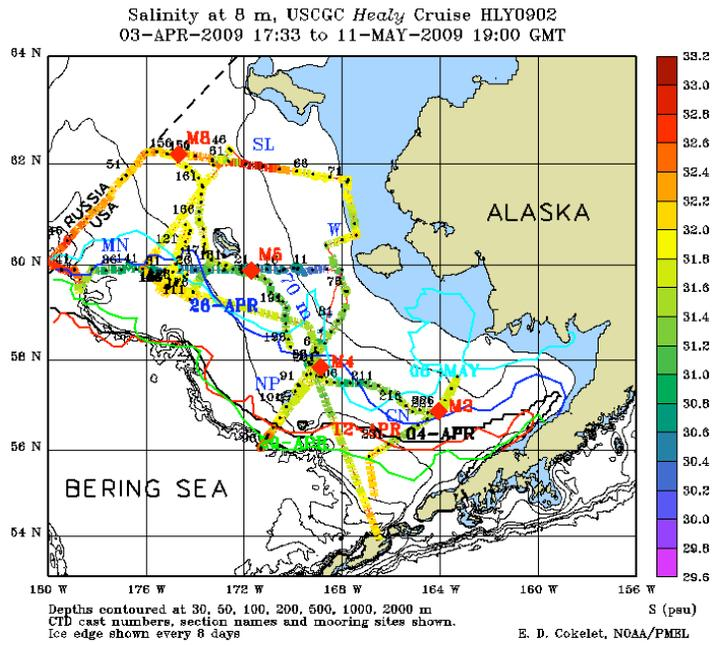
Figure 3. Salinity at 8 m depth measured by the underway seawater sampling system.
