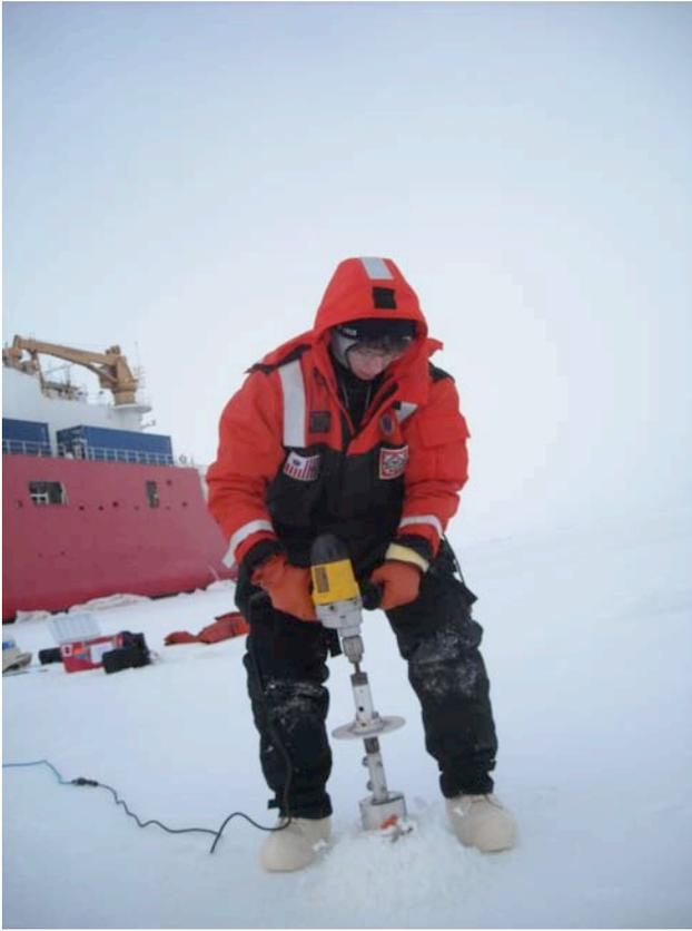
*H. Chenelot (UAF) takes an ice core in thick sea ice. If sea ice thickness exceeds core length, an extension has to be added to the corer.*
