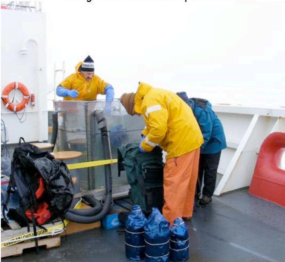
Figure 1. Ashjian/Campbell plankton wheel incubator, showing incubation bottles wrapped to simulate 15% in situ light level being placed on the plankton wheel. Bottles are slowly rotated for a 24 hour period while being immersed in flowing water at near surface seawater temperatures.
