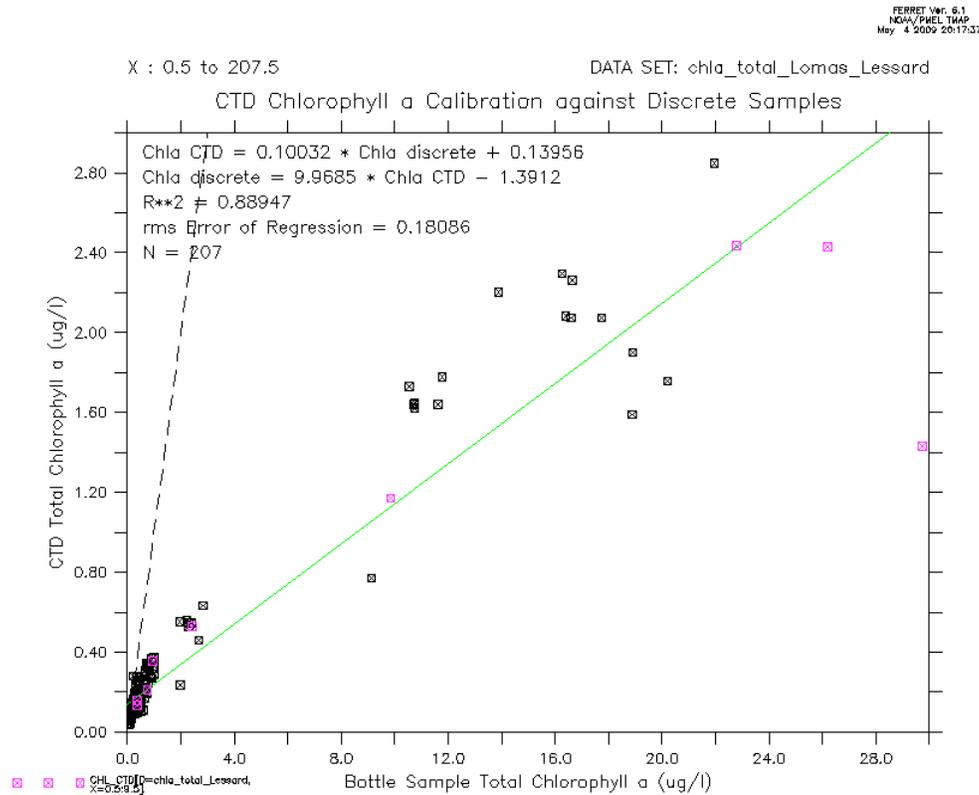
Figure 1. Linear least-squares-fit field calibration of the CTD fluorometer.
