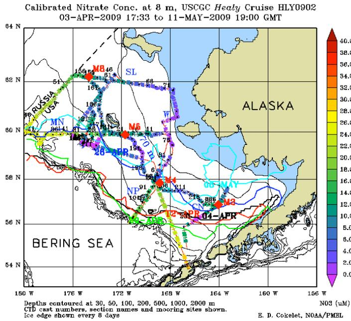
Figure 4. Calibrated dissolved nitrate concentration at 8 m depth measured by the underway seawater sampling system.
