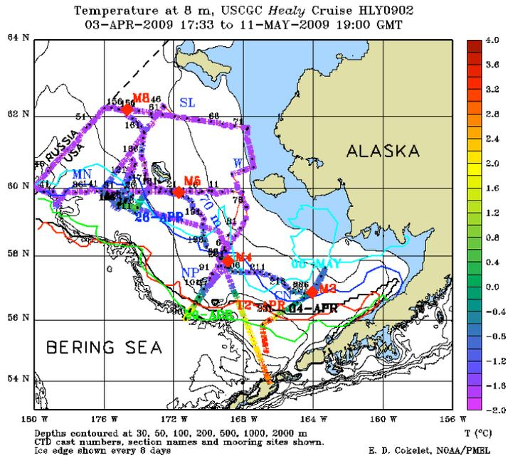
Figure 2. Water temperature at 8 m depth measured by the underway seawater sampling system.
