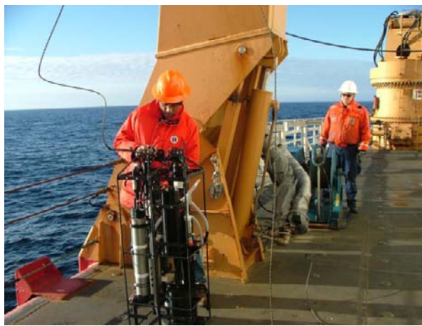
Figure 1: Bio-optical package before deployment at a station in the Bering Sea during USCG Healy cruise 0803.
