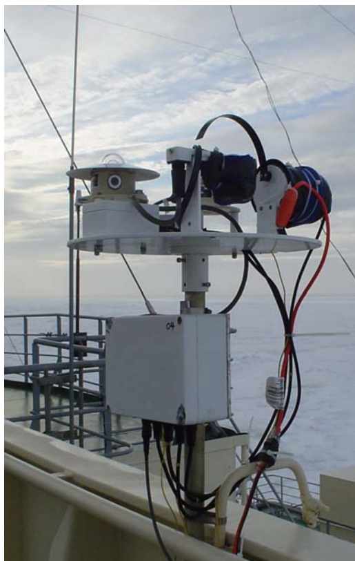
Figure 4 Portable Radiation Package on the I/B Kapitan Dranitsyn . above the bridge of the I/B
