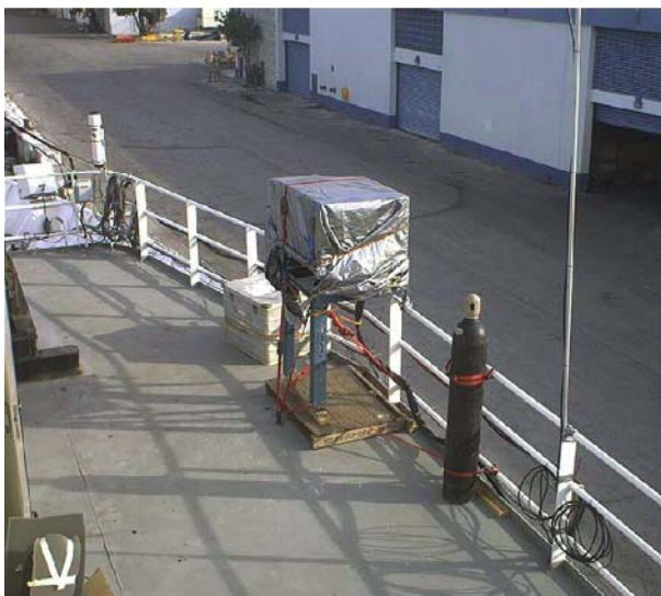
Figure 1a. M-AERI mounted on starboard side railing on the O2 deck of the Ronald H Brown . The instrument is covered by a tarpaulin, which is the case when there is heavy rain or sea-spray. Measurements are not taken while covered.
