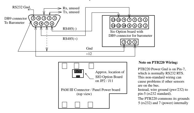
EVE communicates with the PTB220 using a poll command that is distinct from the Sbus message protocol defined by NCAR. Likewise the barometers must ignore all other messages that are not addressed to them. The EVE configuration file declarations for RS485 communications:
