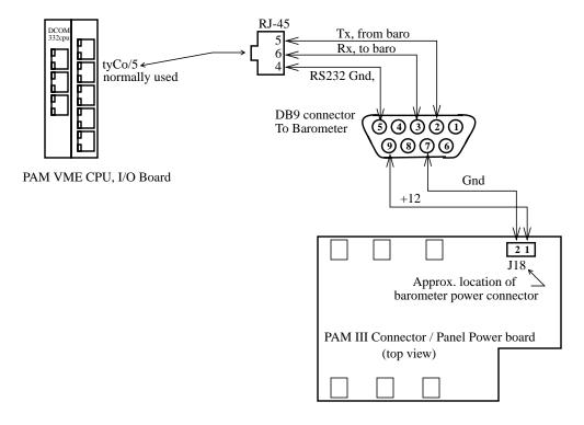
With RS232 Operations, more reliable operations can be expected. The barometer can be operated either in polled, or in automatic message output modes. The sensor baud rate can also be reduced to help improve data system interrupt handling margins, however for convenience it is probably better to retain the same baud rate as with RS485 to prevent confusion when switching back and forth between methods.
