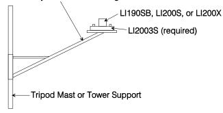
FIGURE 2-1. 015 Pyranometer Mounting Arm
