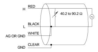
FIGURE 3-1. LI200X Schematic
