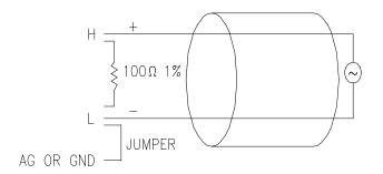
FIGURE A.2-1. Unmodified Pyranometer Wiring Schematic
