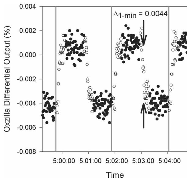
FIG. 2. Example of the Oxzilla differential  $O_2$  signal over several 1-min switching cycles, while comparing two reference gases. The vertical gray lines indicate the time at which the changeover valve is switched and open circles show data that are ignored after each switch. In this case the gases have an apparent  $O_2$  mole fraction difference of 0.0022%, which results in a signal amplitude of 0.0044% because of the crossover switching arrangement.
