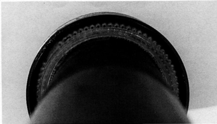
Fig. 4. End-on view of inlet manifold. Aerosol sample is injected through small holes between two rows of sheath air holes.
