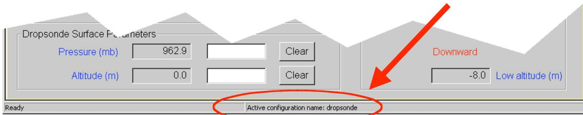
The initial installation of Aspen provides a configuration set named “dropsonde”, and designates it as active. These parameters are generally useful for dropsonde soundings in a tropical environment. If analyzing dropsonde soundings in different environments, as well as upsonde soundings, you will almost always need to create a new configuration set and adjust its QC parameters appropriately.
