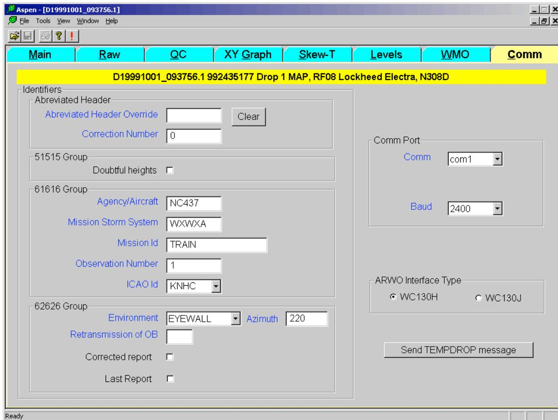
The Comm tab is used to enter the administrative information that is coded in the WMO message. It also has controls for transmitting the WMO message via an attached interface on the USAFR WC130 aircraft. The field names should be self-explanatory.
