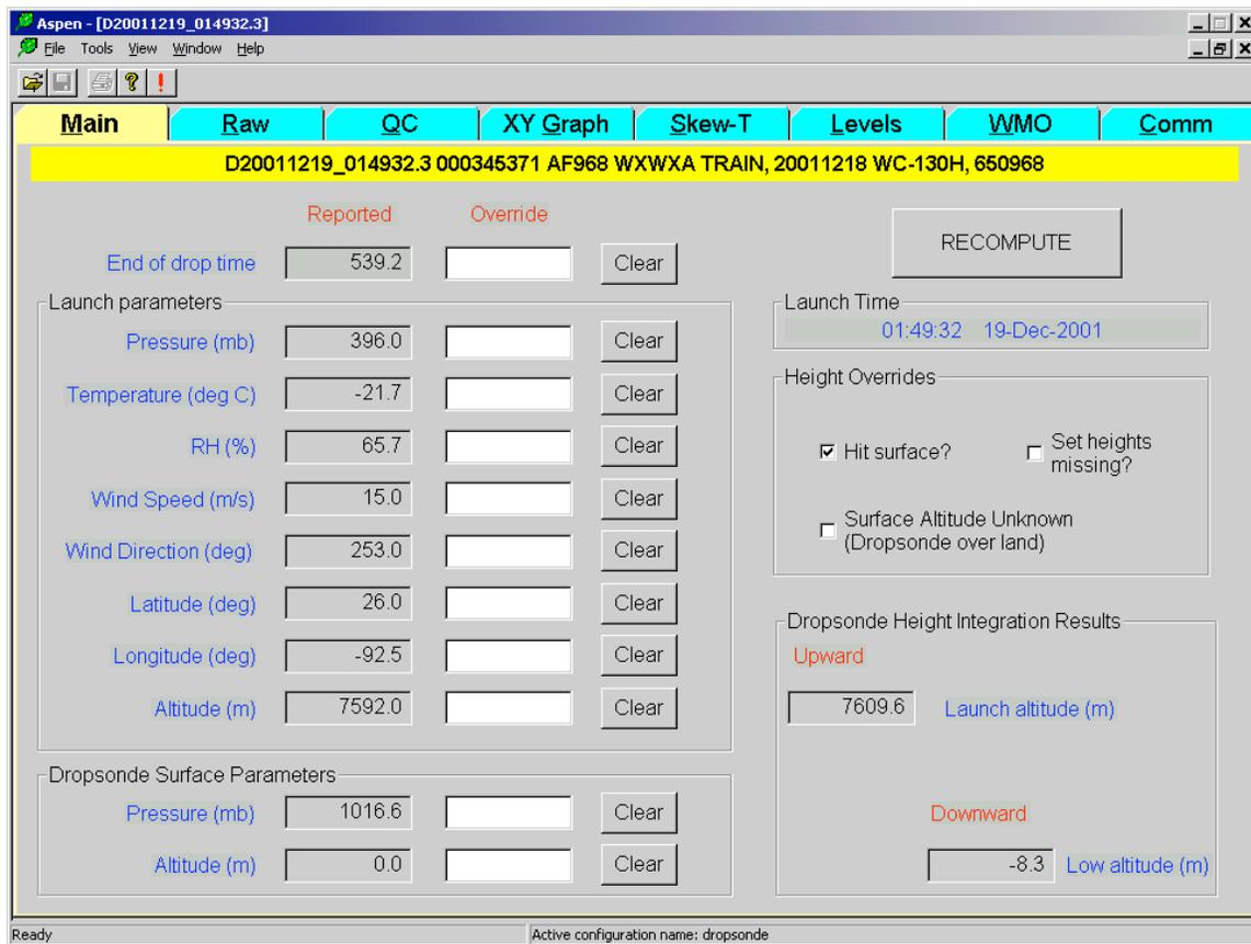
The Main tab is used to specify certain characteristics of the sounding, and to override the launch point observations. Entering a value into the appropriate box specifies the override. To remove the override, press the associated Clear button.
