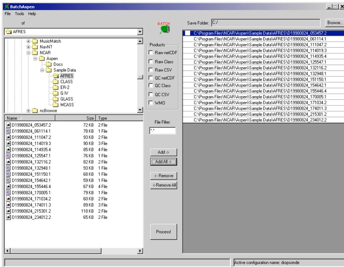
On the left side, there are two independent directory browsers, either of which can be used to navigate into directories containing input files. The files in the selected directory are shown in the file selector in the lower left. The display of file types can be restricted using the “File Filter” in the center edit box.
