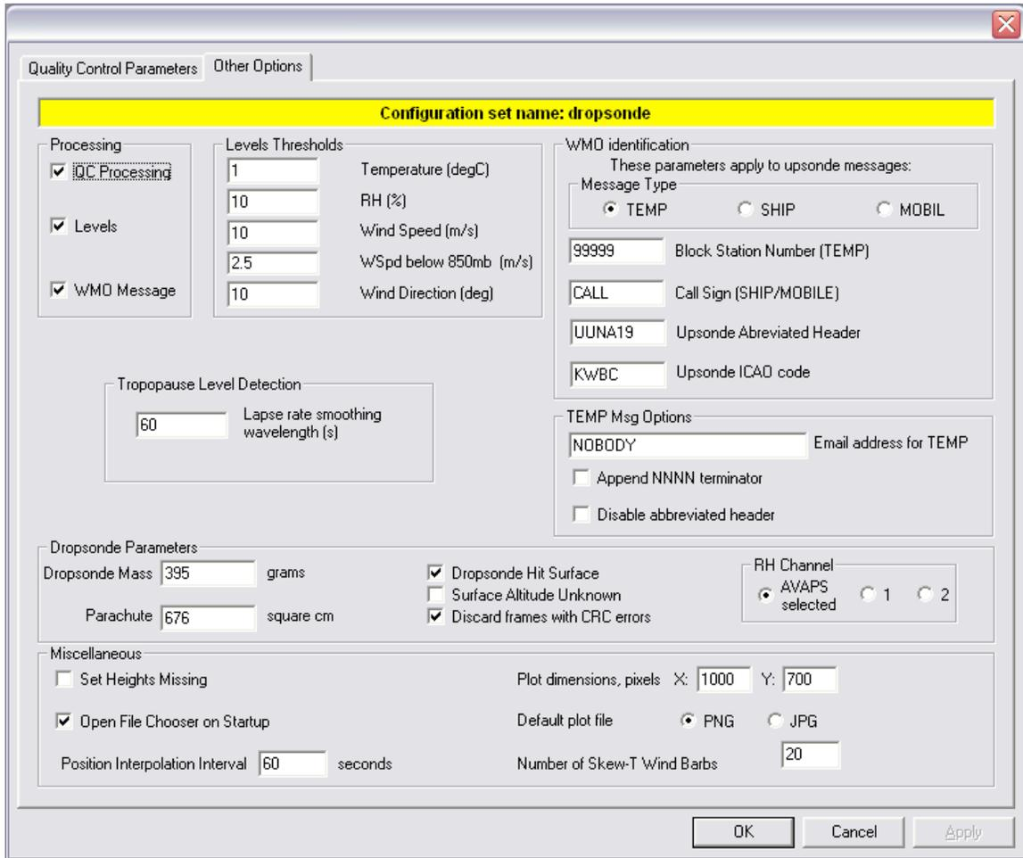
**QC Processing.** In normal usage, this feature should always be enabled. If it is turned off, Aspen will only display the raw sounding data. This may be useful if you want a quick look at a large data set without waiting for processing.
