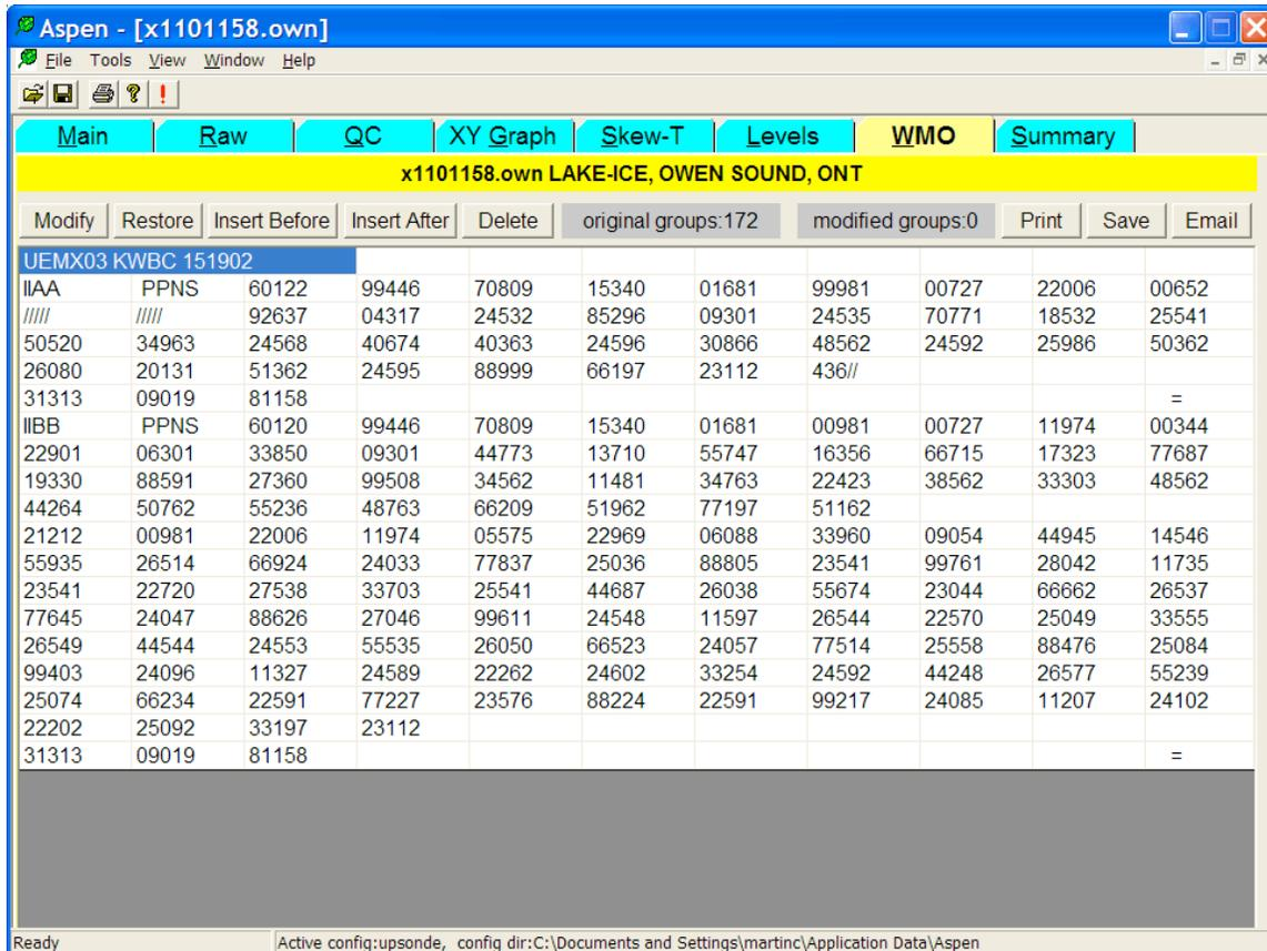
The WMO tab displays the WMO message, which has been coded from the levels information. It can be previewed and printed from the File menu, and also saved as a text file using the *Save* and *Print* buttons.
