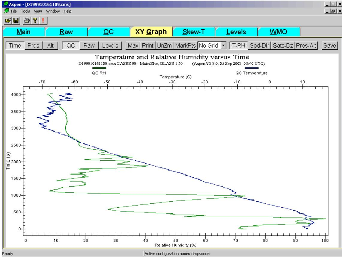
This tab provides numerous options for graphical display of the data. The buttons above the graph select which data products and parameters are displayed. The buttons also select the choice of vertical axis. The main options on the XY Graph tab are as follows:
