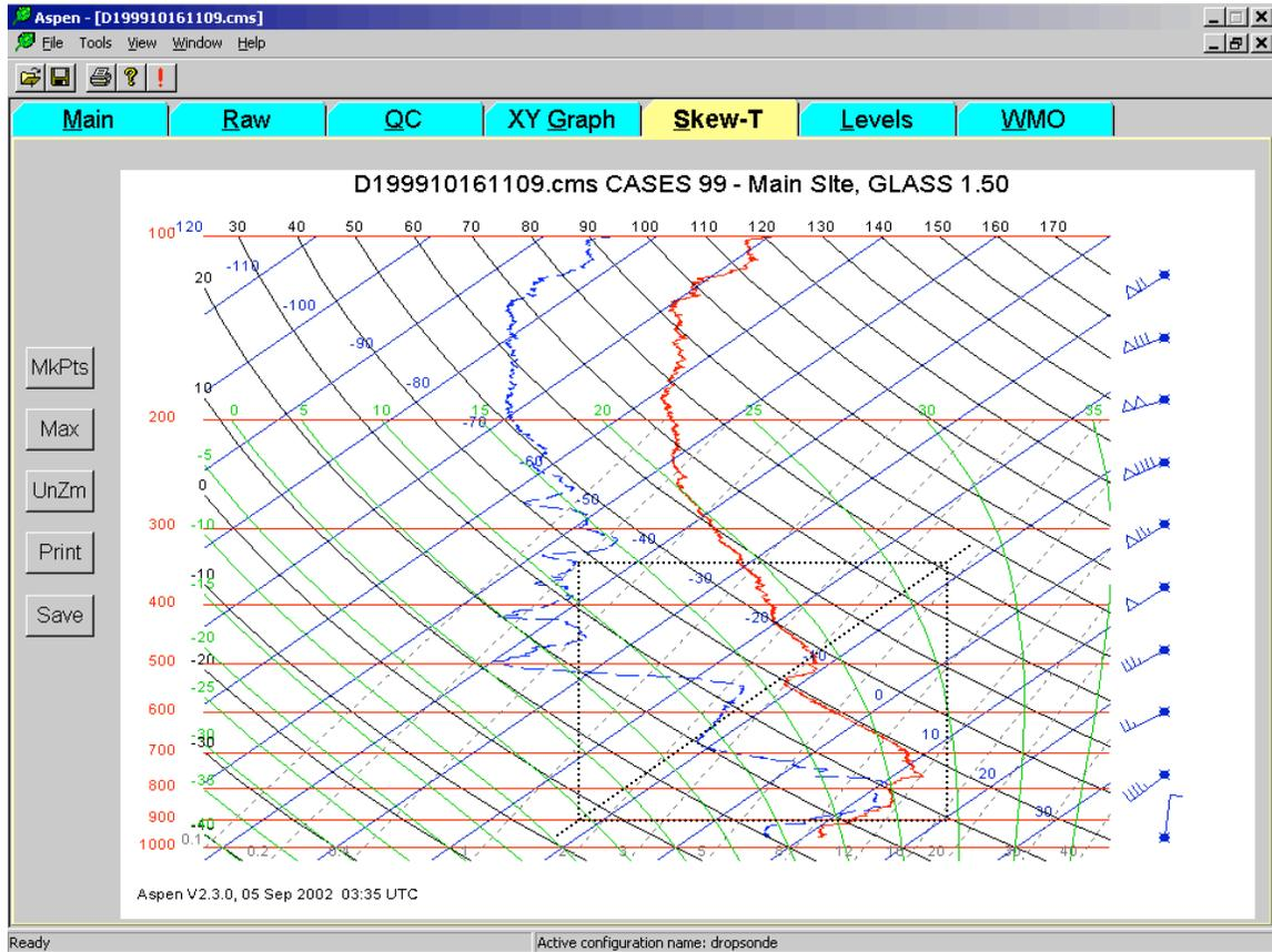
A standard skew-T log-P plot is accessed in the Skew-T tab. Zooming, maximizing, printing and saving of the plot are available in the same manner as for the XY Graph. The right mouse button brings up the same menu of plot options as well.
