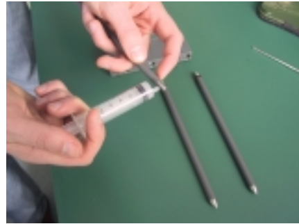
4) put silicon grease to the threads of the rods (new spare rod are greased at works)
