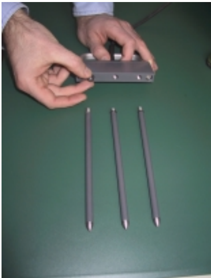
2) put the seals into the borings
