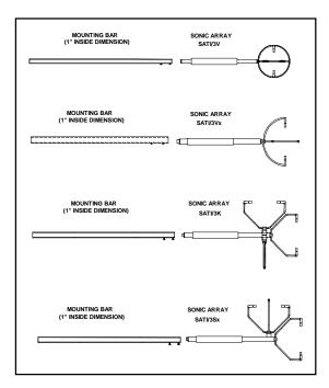
The "Sx" style probe is also available in a one or two axis array. The "K", "V" and "Vx" style probes are strictly three axis probes. All probes are constructed of solid aluminum arms, sufficiently small enough to minimize any cross-sectional area exposed to the wind flow being measured. A transducer is mounted on the end of each arm. These transducers operate in both a transmit and receive mode.
